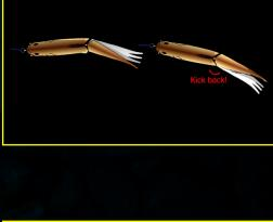
suppresses the noise generated by the collision of the joints, but also creates a lively wave by the secondary action generated by elastically pushing the rear body back. **WATER THROUGH DUCT**
