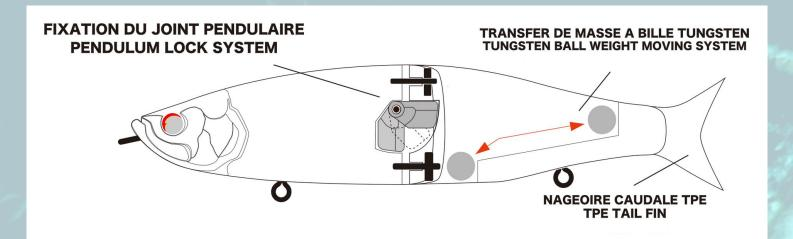
It is relatively easy to control the range of motion of the joints during flight. However, the range of motion is restored at the same time as landing on the water. This part was a big problem.
